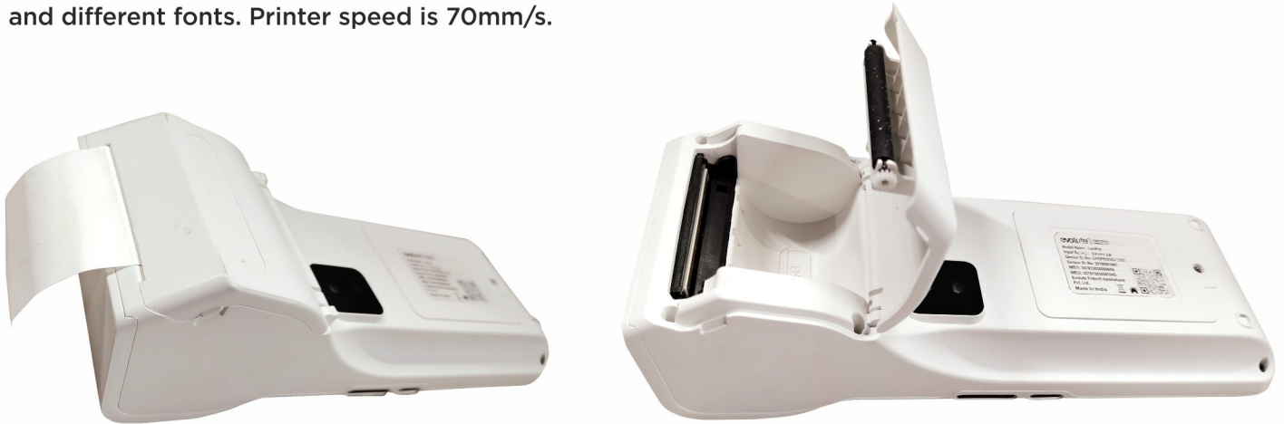
Fig : Printer door open and cabin to place paper roll
